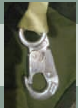
Left: An adjustable lanyard for fall safety and positioning on towers. Above: A double-locking lanyard clip.
