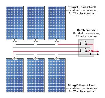
A **string** is a grouping of modules wired in series. Basic electrical physics tells us that connecting electrical sources in series increases voltage, which is exactly the goal of a string. It's the same as when you put three D-cells into your big flashlight—they are in series to attain higher voltage.
