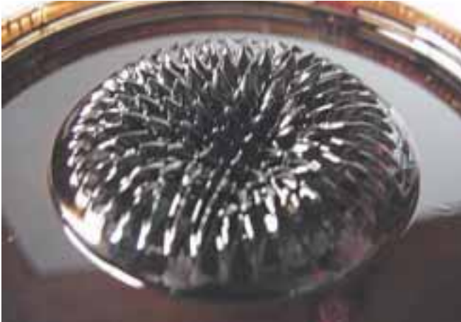
There is a magnet below this dish full of ferrofluid— what we're "seeing" is the magnet's field.
