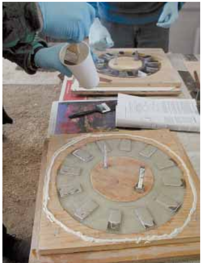
Close-up of students casting magnets in resin during SEI’s Homebuilt Wind Generators workshop.
