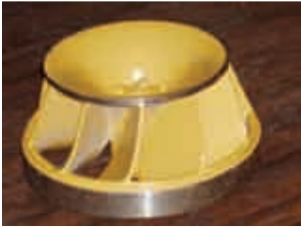
This Francis runner is an example of a reaction turbine, which is submerged in water and rotates with the force of water flowing through the equipment.
