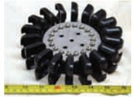
In a Pelton runner design, water impacts the wheel's spoons parallel to the plane of rotation.
