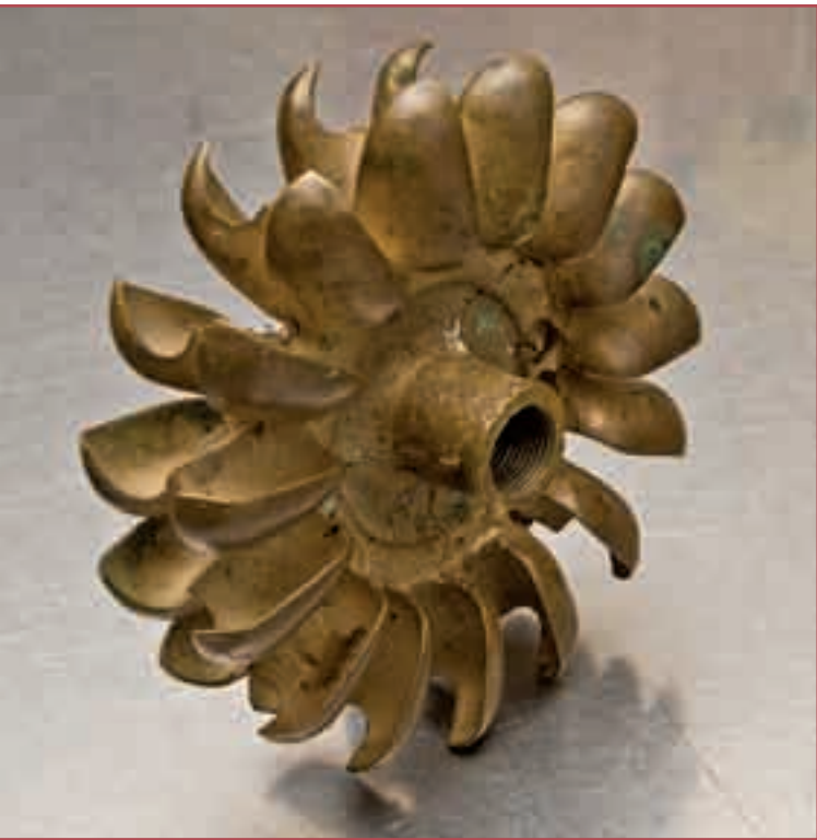
The double-cup design of the Pelton runners is best for a very high head-to-flow ratio.
