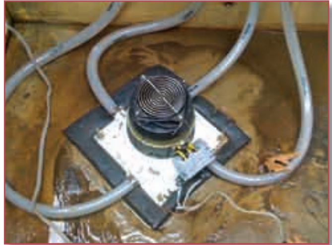
Four different-sized nozzles on this turbine allow 15 possible combinations of flow and power.
