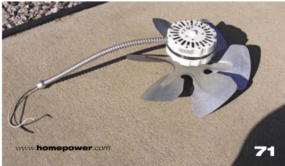
One of the two inefficient electric attic fans that were removed and replaced with ridge and soffit vents.
