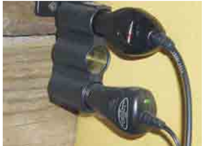
Cigarette lighter receptacles are the most common 12-volt DC receptacle, but they have multiple problems.
